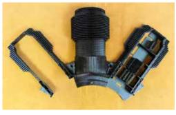
Left: One half, 3D printed, cylinder head. Right: One complete and two partial cylinder halves give an idea of how things will go together.
